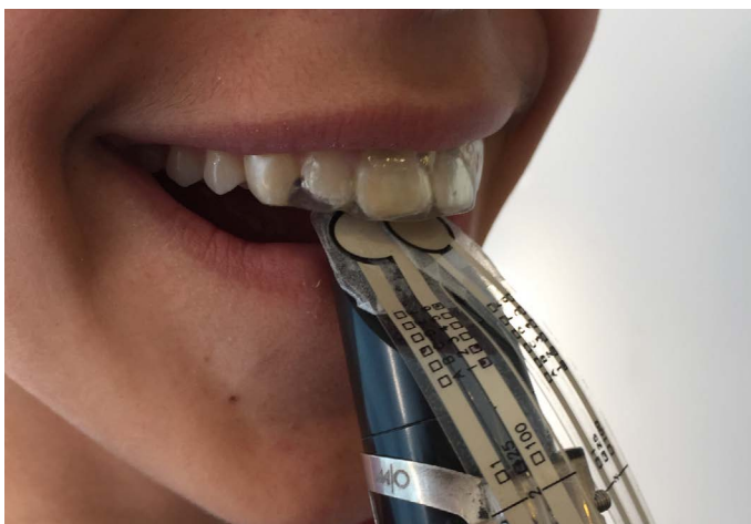
Figure 5. Evaluation of the tooth pressure with the Flexiforce sensors while wearing the homemade ESMA device
