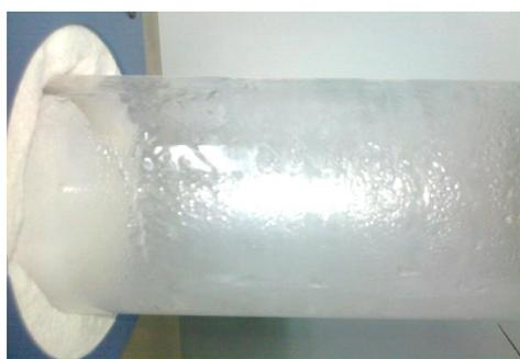
Figure 2. Water condensation outside of quartz tube
