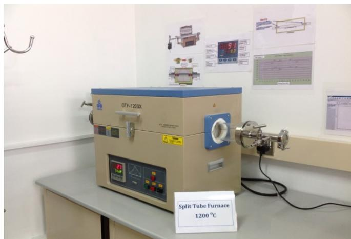
Figure 1. Split tube furnace
