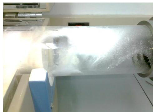
Figure 5. Quartz tube all inner surfaces contaminated
