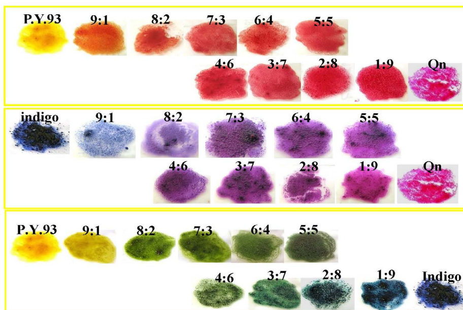
Figure 12. Multi-colored micro-capsules prepared by mixing three primary colors of latent pigments
