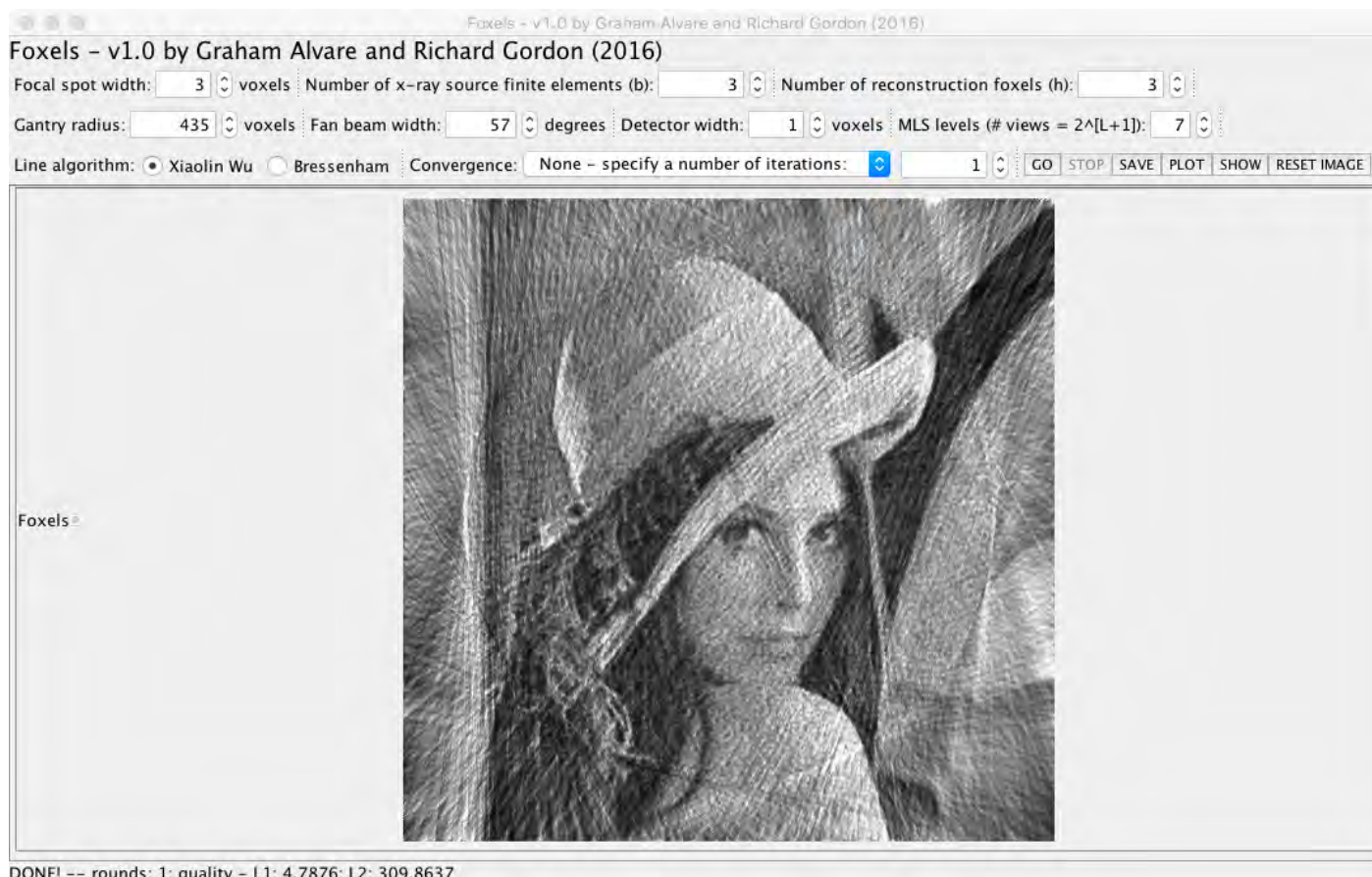
Figure 11. User interface. The FoxelCT user interface is shown after selecting the image to reconstruct, with output shown at one iteration (“round”). The input image is converted to gray scale if it is a color image. The Bresenham “staircase” algorithm for drawing lines[256] was not explored for representing rays in this paper. Alternate convergence (stopping) criteria are: variance method, Q_1 and Q_2 , but the calculations can be continued after stopping. A log of all the input and output parameters and the current reconstructed image can be output by the SAVE command. The PLOT shows the voxel values along a horizontal line through the center of the latest reconstructed image. The SHOW command may be used to display the original input image. However, after clicking SHOW, except for the information in the log, the work done so far is lost. RESET IMAGE deletes the work done so far (except for the log text), allowing a start from scratch. It can be useful when comparing the effects of different parameters on a single image. STOP ends the program with the image that is currently displayed on the screen. That image is updated after every iteration, so the progress of the computation can be followed visually. The file name convention for the output we use in this paper is just the parameters in the order shown here, namely “Lena 3 3 3 435 57 1 7 W 1” in this example. Note h = a_w . In terms of our equations, the values in the first two input rows correspond to f_w, \psi_w, a_w, r, \Phi, d, G = 2^{L+1} .
